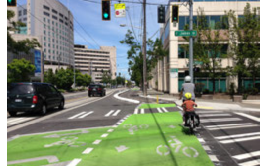
An early signal phase for bicyclists reduces conflict with turning vehicles, while use of green defines the infrastructure and increases awareness of conflict zones.
