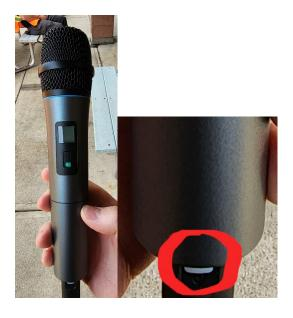
If it does not turn on it means that the battery is dead. To swap batteries twist the bottom of the handheld and remove the batteries.
